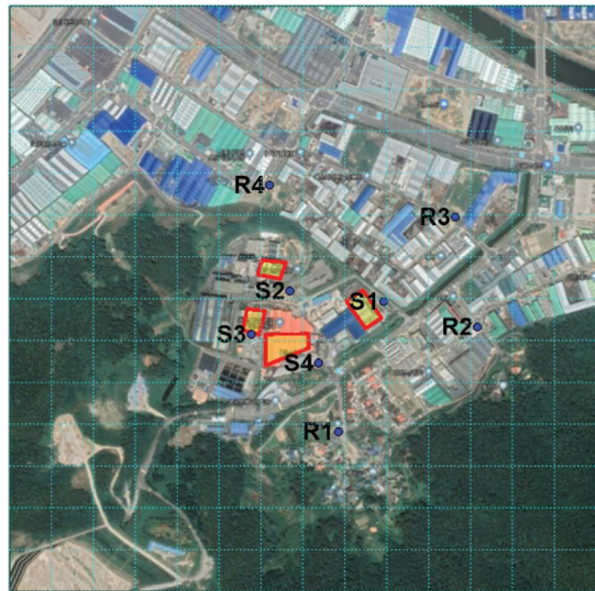
Fig. 2. Geographical map of modeling domain including locations of 8 sampling sites and 4 area sources, S1 to S4 and R1 to R4 are the locations of complex odor sampling sites used for model result verifications. The red rectangles are the locations of area sources considered in this study.
